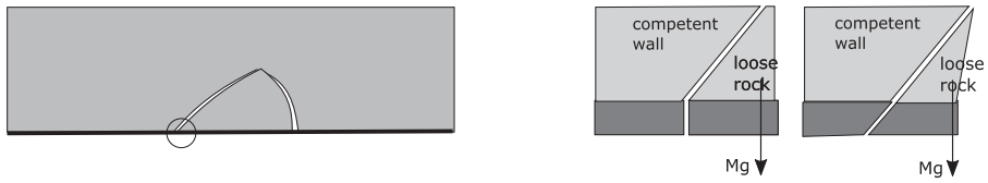
FIGURE 5. Failure through liner rupture. Left: The supported rock. Right: A close up of the situation near the rupture point (circle). Two liner rupture modes are possible: shear failure and tensile failure.
