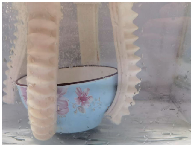
Figure 14. Gripping experiment: The soft gripper without spring steel plates was broken.
