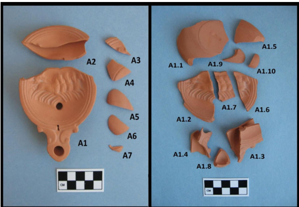
Fig. 8. Lamp A sherd generation after Stage 1 (left) and Stage 2 (right) drop experiments. The sherds were arranged by the author for clarity. (E. Lapp.)
