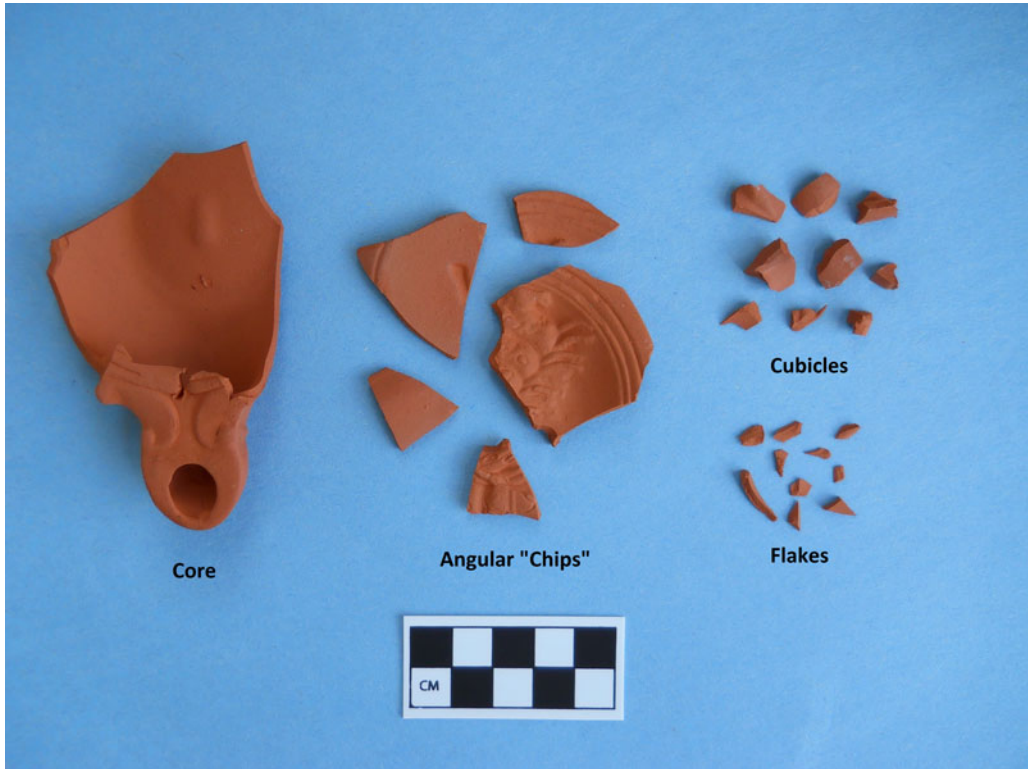
Fig. 7. Types of lamp sherds generated from drop and impact experiments. (E. Lapp.)
