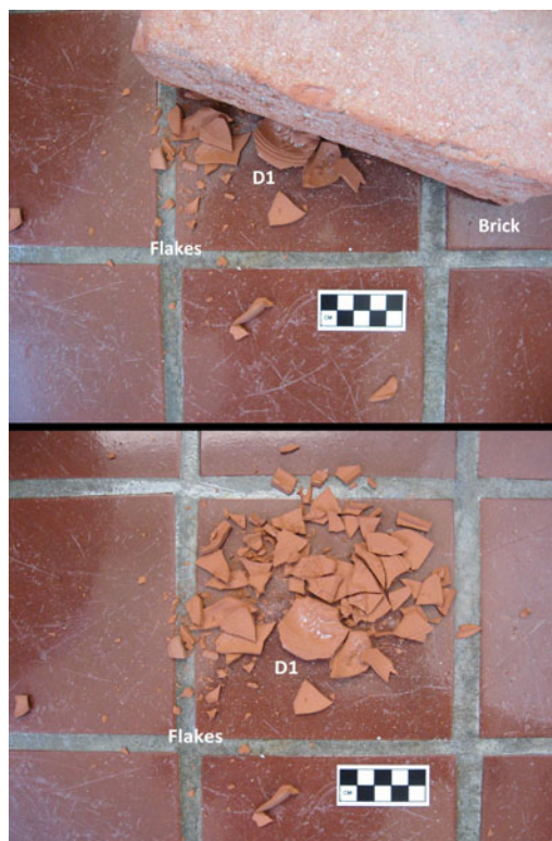
Fig. 13. Concentrated sherd pattern resulting from impact experiment conducted on Lamp D. (E. Lapp.)
