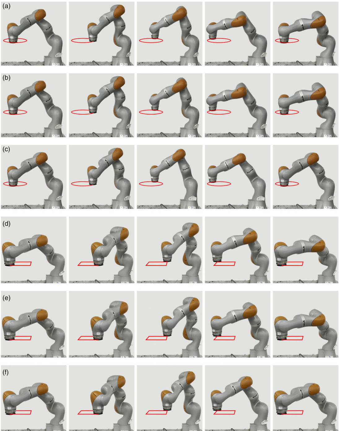
Figure 7. The experiments for tracking the circle (first three rows) and square (last three rows) paths are performed on the KUKA manipulator using (a), (d) KDL, (b), (e) TRAC-IK, and (c), (f) the proposed algorithm, respectively. The KUKA manipulator begins with the initial point (first column), moves counterclockwise through the path points (middle three columns), and finally gets back to the start point (last column).
