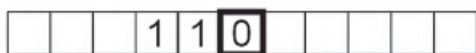
Figure 1 A simple Turing machine that flips each 0 into a 1 and each 1 into a 0
