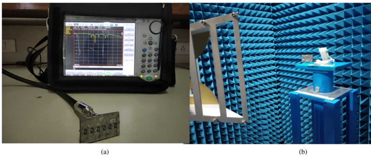
Fig. 5. Antenna under test at (a) Anritsu Site Master, S820E VNA (b) Anechoic Chamber for testing antenna radiation pattern and gain.
