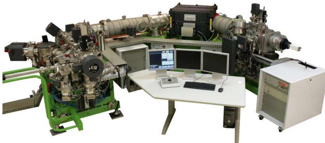
Fig. 1. Cameca ims 1280 ion microprobe. The primary ion column is on the left, the sample sits behind the round gray cover just to the left of the table, and the secondary-ion mass spectrometer extends from the sample in a U-shape to the right. The magnet for the mass spectrometer is in the large gray box above the table.
