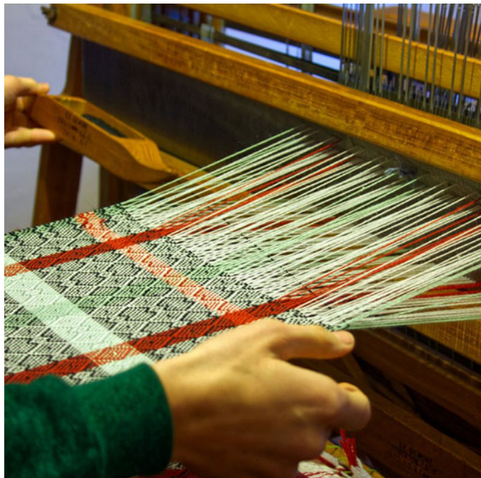
Figure 10: A loom with red, green and white yarns used in both the warp and weft. 23 The configuration of the weft yarn changes with each line according to a pattern.
