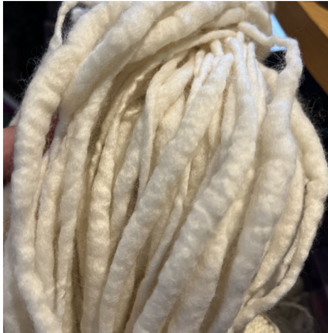
Figure 9: ‘Thick–thin’ yarn. This spun wool has been plied once and felted using moisture and heat.
