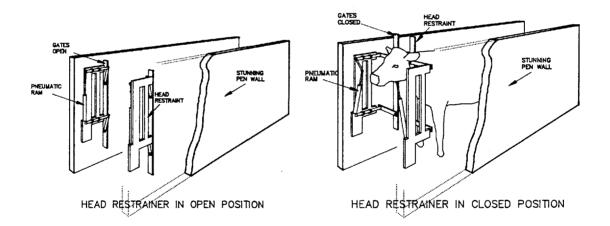
Restraint is by means of two vertical bars which, in the open position are folded back to the inside of the front of the pen. When activated the two bars are pushed, by pneumatic pistons, towards the mid-line of the pen and grip the animal's neck between them. This restricts the movement of the head and should thus make it easier for an accurate stun to be carried out.
