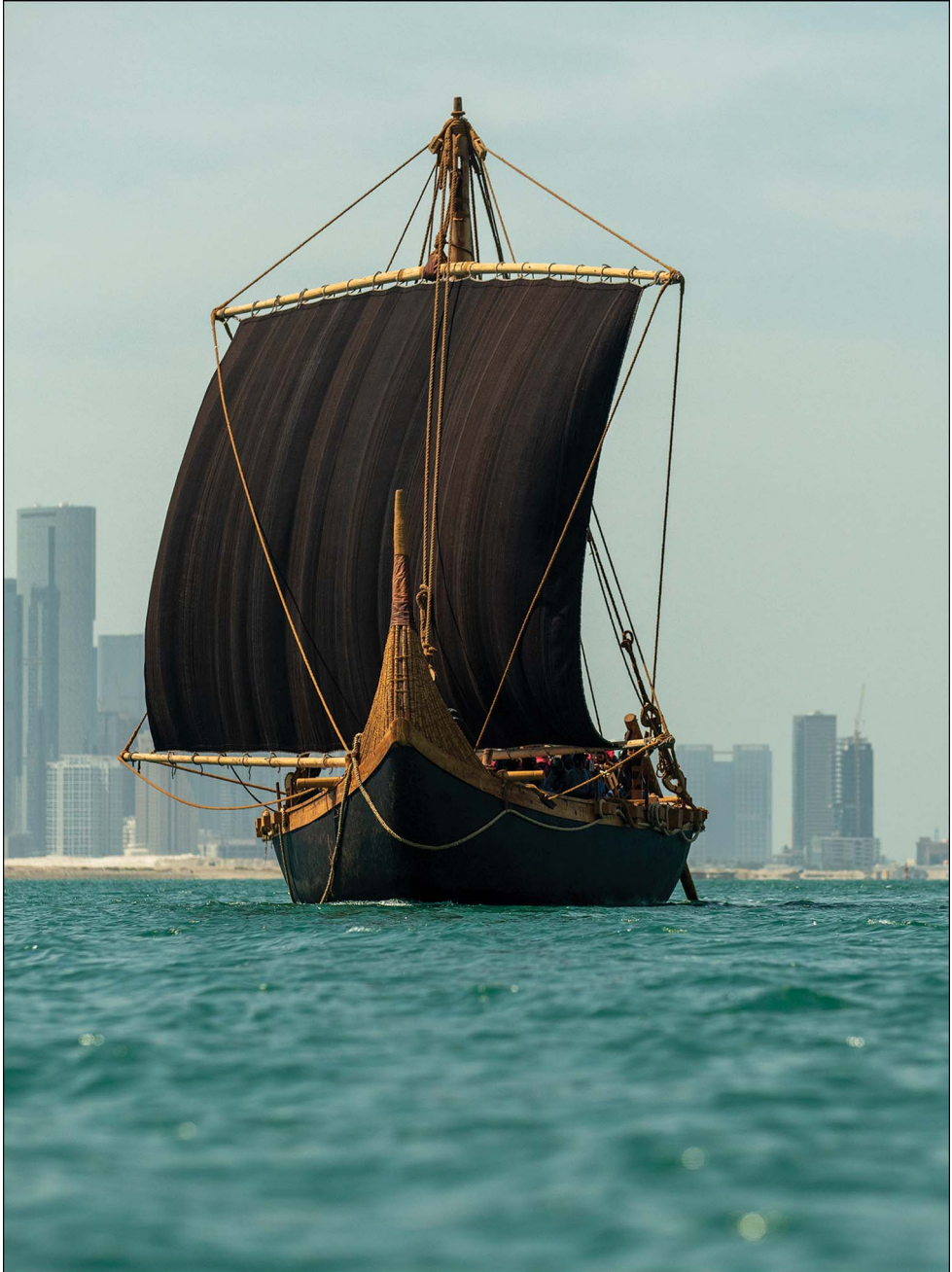
Frontispiece 2. An 18m-long reconstruction of a Bronze Age ship undergoing sea trials off the coast of Abu Dhabi, UAE, in 2024. The vessel was built by shipwrights using traditional tools to a design based on information from Sumerian cuneiform tablets and ancient representations of boats typical of the land of Magan (modern-day Oman and the UAE). The hull of the wooden-framed vessel is made of 16 tonnes of reeds lashed together with palm-fibre rope and coated in bitumen; the sail is made of goat hair. During testing, the vessel reached speeds of 5.6 knots. The 'Magan Boat' is the result of a collaboration between the Zayed National Museum, New York University Abu Dhabi and Zayed University. Photograph by E. Harris © Zayed National Museum.
