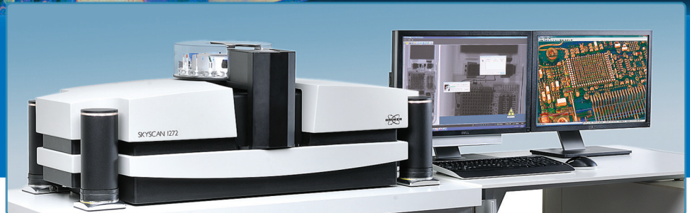
Volume rendering of the internal structure of an MP3 player. 5µm isotropic pixel size, 4904x4904x7491 reconstructed volume
