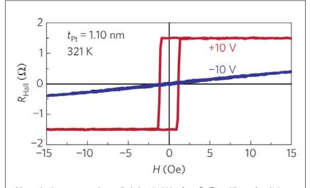
Magnetization curves under applied electrical bias for a Co/Pt multilayer. A switch from ferromagnetic (+10 V) to linear behavior (-10 V) is clearly visible. Reproduced with permission from Nature Mater. (DOI: 10.1038/nmat3130). © 2011 Macmillan Publishers Ltd.
