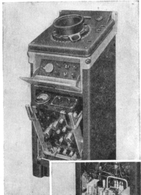
Display Unit— with front panel removed for servicing. Note metering panel for fault location.
