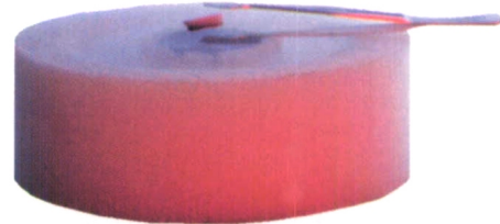
A magnet levitated over a thin film superconductor at LN 2 temperature.
