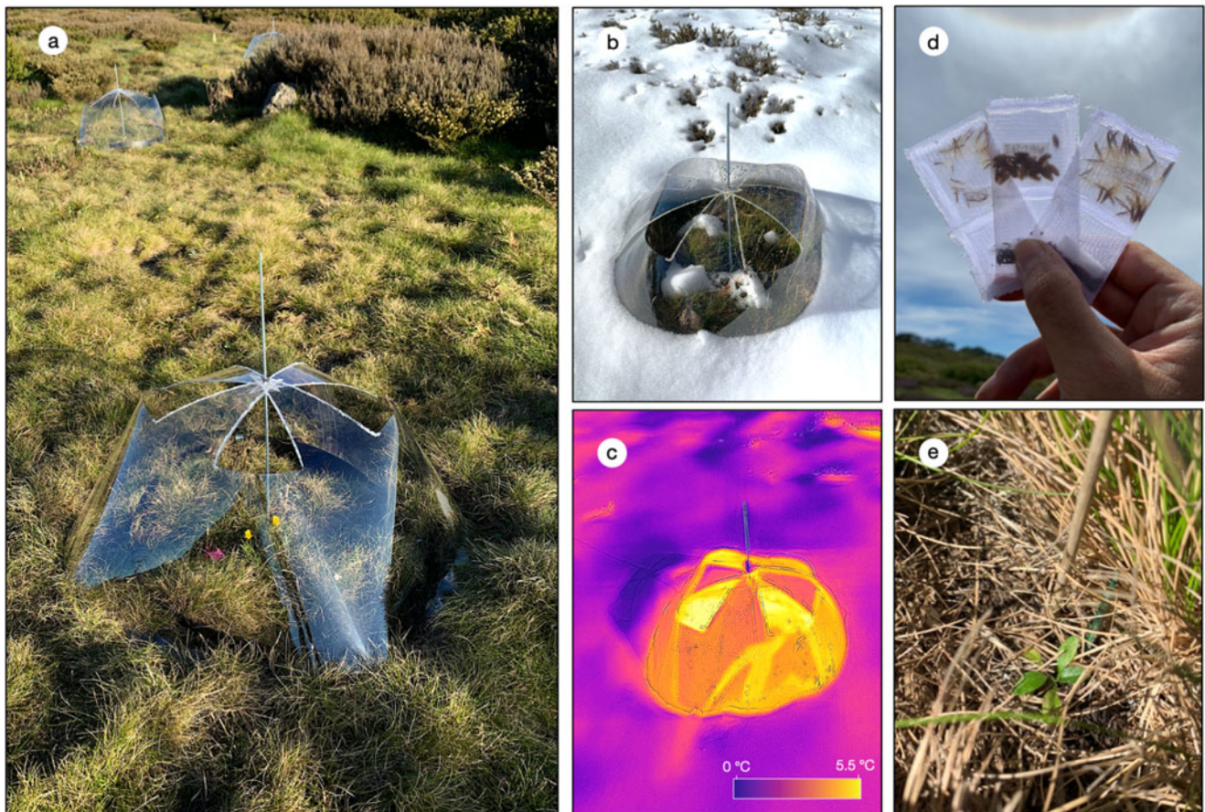
Figure 1. (A) Chambers used during the study, (B) a chamber after a light snowfall demonstrating how any snow inside the chamber melts faster than ambient conditions, (C) thermal image indicating the temperatures inside and outside the chamber and (D, E) seeds and seedling can be sowed within the chambered plots to understand their response to a warmer and drier microclimate.
