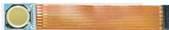
FIG.3. The SDD moutage is very flexible and accounts for the small amount of space available in an electron microscope.
