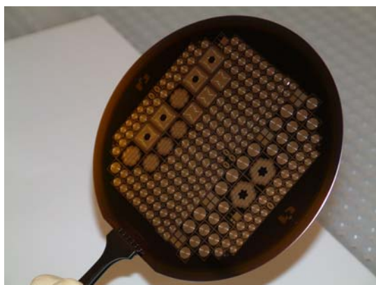
FIG.1. SDDs with integrated FET are fabricated in a monolithical planar silicon process in an ultrapure technology providing excellent energy resolution at high temperatures.
