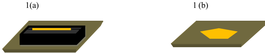
Figure 1(a). Cartoon of mounted cross-section for SEM prior to freeze-fracture of the extended film. Figure 1(b). Cartoon of mounted planar section for SEM.
