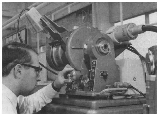
Figure 2. Dr. Jenkins setting up one of the first X-ray spectrometers at the ESSO Research Laboratories.
