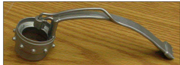
Figure 3. Fuel circuit made by direct metal additive manufacturing.
