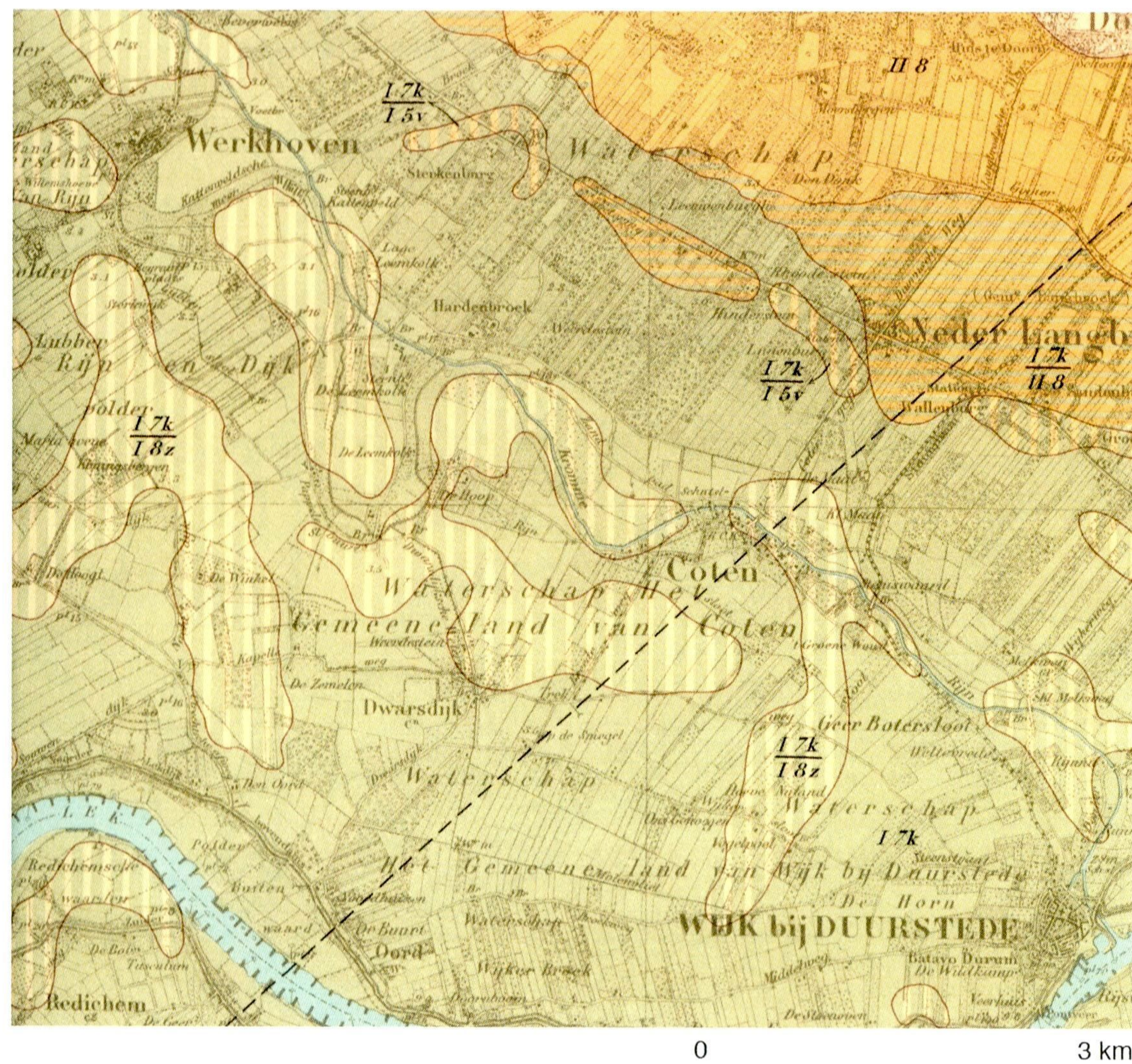
Fig. 2. Fragment of the first geological map, scale 1 : 50,000 of the Netherlands (Tesch 1936). Note the 'islands' of sand (code 17k/18z) that are actually parts of channel belts. Green (code 17k) = floodbasins.
