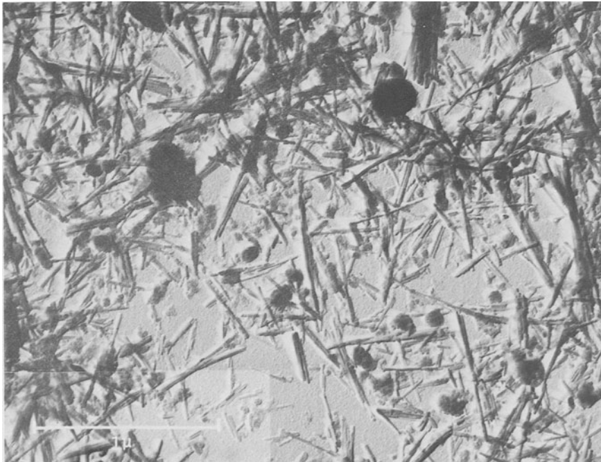
Fig. 4. Electron micrograph of fine clay for which the X-ray diffractogram is shown in Fig. 2.
