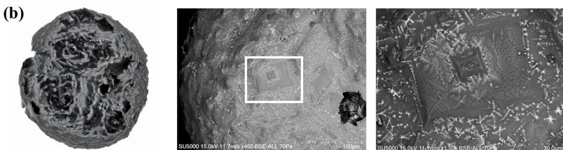
Figure 2. (a) OM of a typical barred olivine MM with a table of EDS-measured elemental composition by weight % [1] that indicates chondritic composition when compared by element/Si ratios to MMs obtained from the Antarctic [3]. (b) OM of a ~700 µm porphyritic olivine MM found at Nesodden, Akershus, Norway, with BSE micrographs indicating dendritic magnetite formation (bright features).
