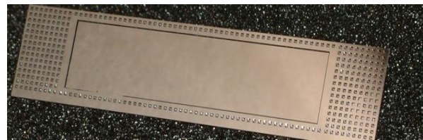
Fig. 3: High purity silicon detector thinned down to a thickness of 50 μm. The detector properties remain unchanged [3].
