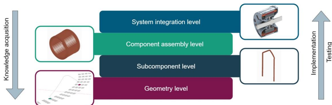
Figure 3. Breakdown structure of the approach given for the example of a hairpin winding
