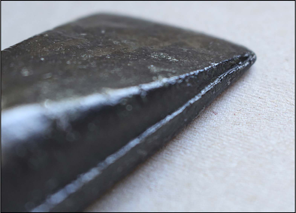
Figure 3. Mould shift on axe 24 (photograph by J. Baron).
