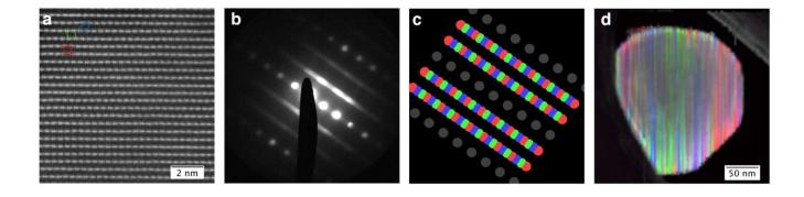
**Figure 1.** (a) HAADF STEM image of LRTMO cathode particle (b) Summed CBED pattern from the 4D STEM dataset, (c) location and shape of virtual apertures corresponding to the three variants and (d) Reconstructed virtual dark field image showing the domains corresponding to the three monoclinic variants in red, blue and green.
