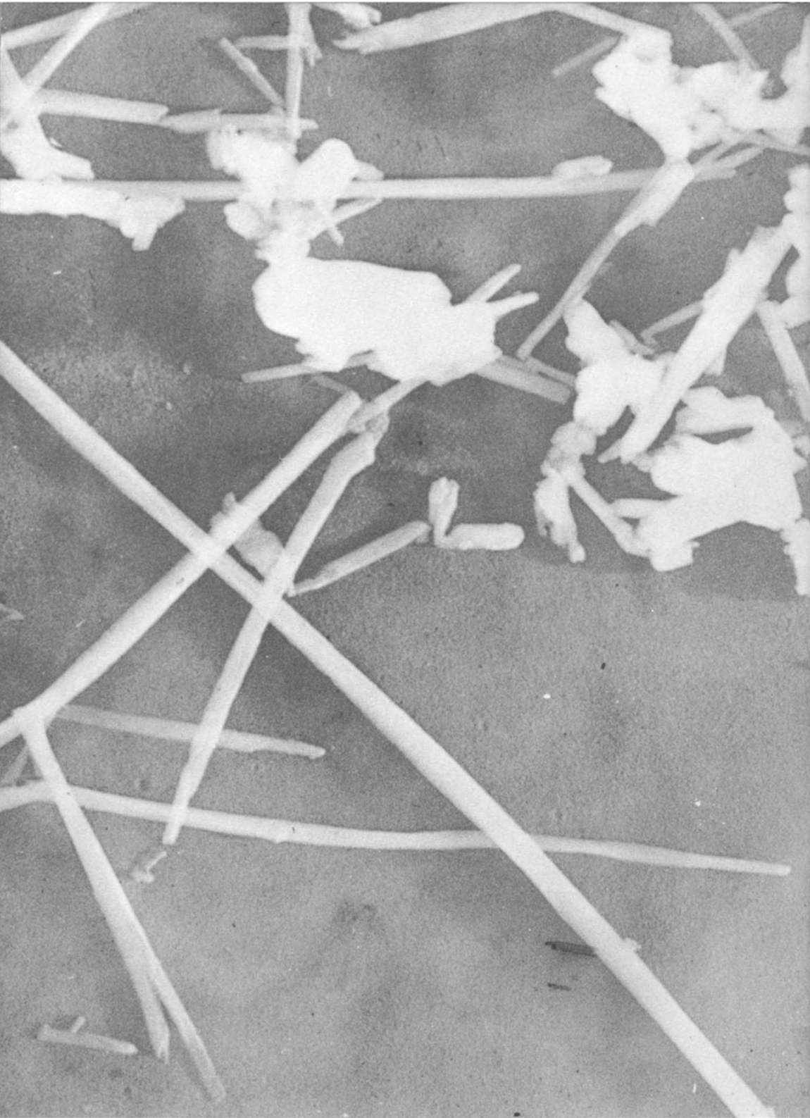
FIGURE 11. — Halloysite. A.P.I. No. 51. Spruce Pine, North Carolina. Magnification: 33,000. (1 mm. = 300 Å.)
