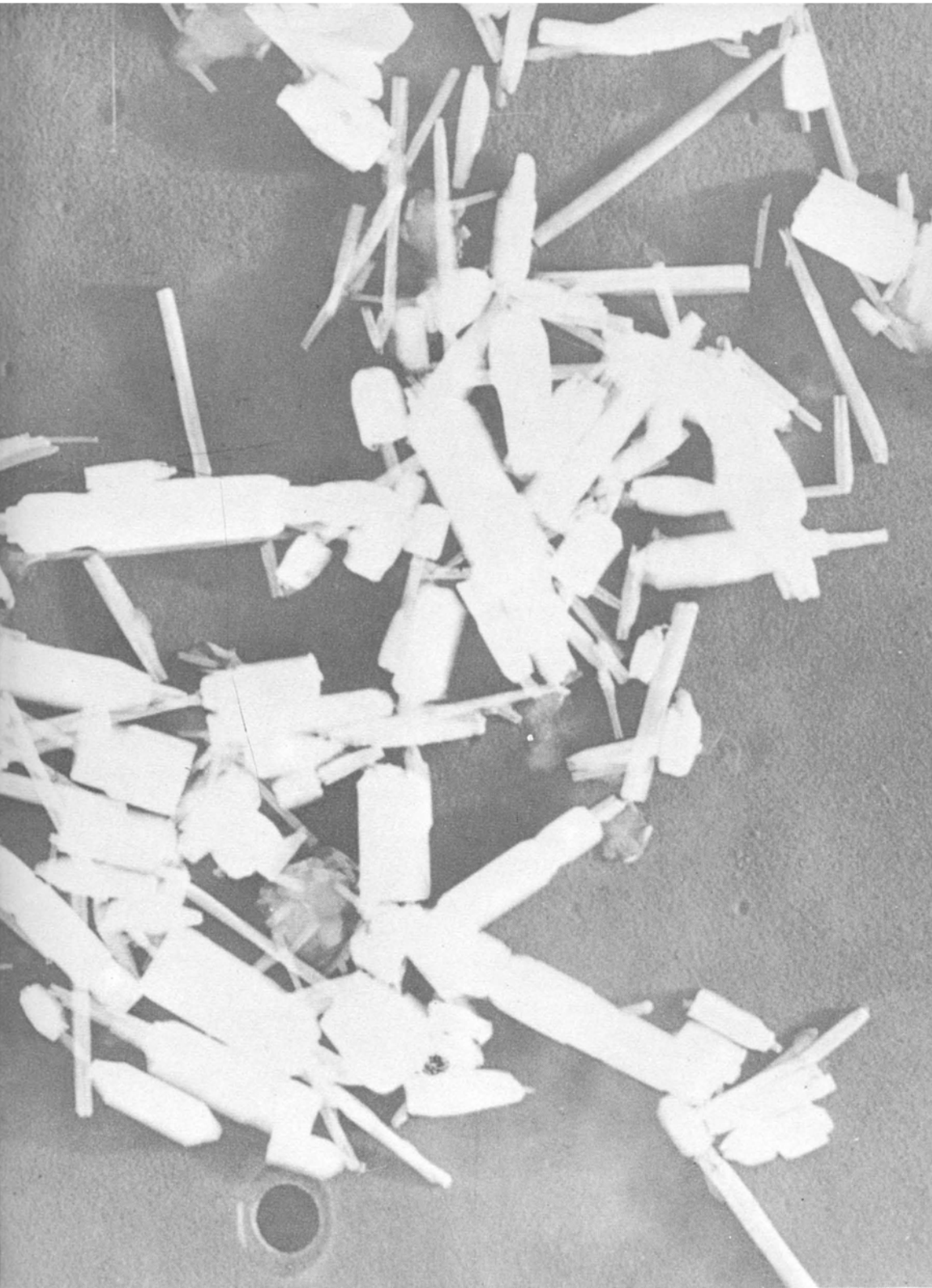
FIGURE 14. — Halloysite. Silver City, New Mexico. Magnification: 33,000. (1 mm. = 300 Å.)
