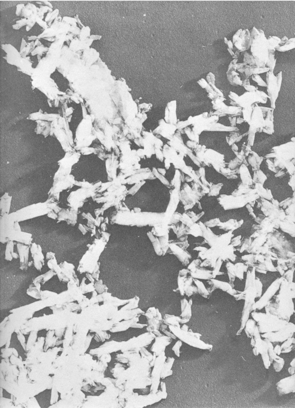
FIGURE 10. — Halloysite. A.P.I. No. 12a. Bedford, Indiana. Magnification: 33,000. (1 mm. = 300 Å.)
