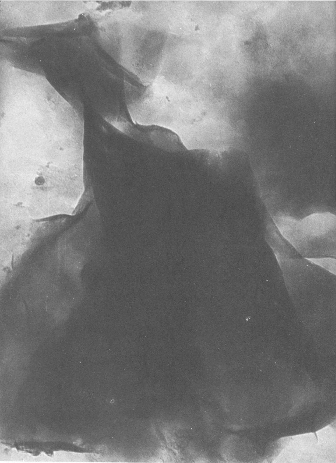
FIGURE 19.— South Texas Outcrop. Manning formation (surface). Magnification: 80,000. (1 mm. = 125 Å.)
