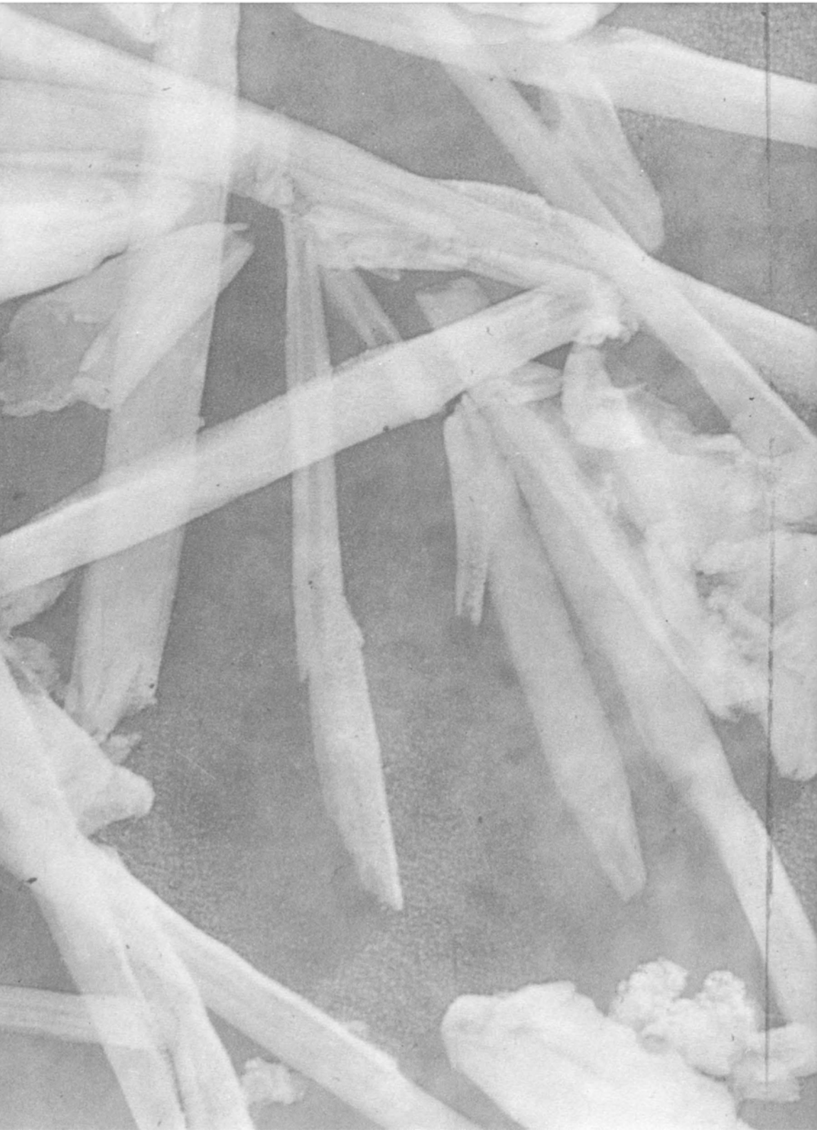
FIGURE 13. — Halloysite. A.P.I. No. 51. Spruce Pine, North Carolina. Magnification: 132,000. (1 mm. = 75 Å.)
