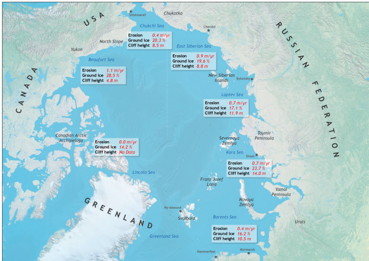
Figure 8.17: Coastal erosion rates at selected sites in the Arctic
