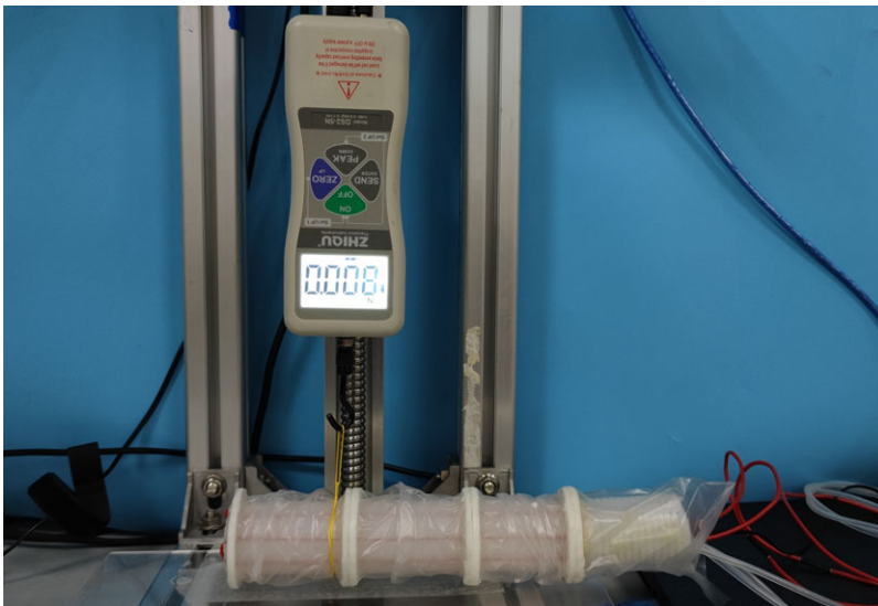
Figure 8. Force test bench for bending of the self-repairing soft actuator.
