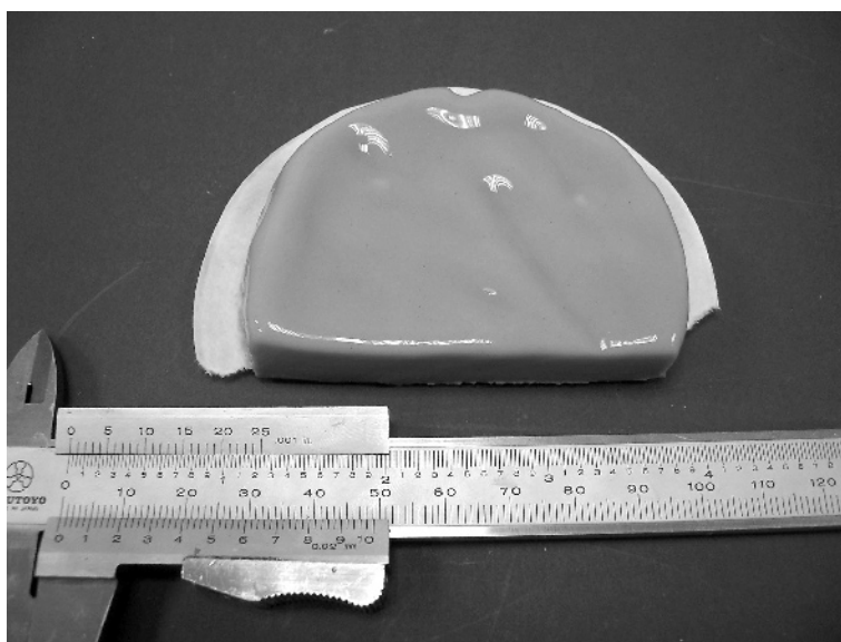
Figure 2. Photograph of a bentonite filter cake showing an indistinct and uneven slurry–cake interface at the top despite careful handling.
