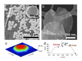
Figure 1. SEM images of platelet-like particles on top of a substrate (a) and on top of a TEM grid (b) and inset in a. AFM 3D image of a single platelet (c). The thickness profile at the centre of the platelet is displayed in d: the measured thickness is 69.4 nm and several steps are observed on top, the smallest measured step has a value of 3.1 nm
