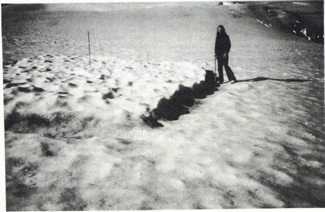
Fig. 3. Experiment performed in the accumulation zone of Blue Glacier on Mount Olympus, Washington State, U.S.A., in July 1980. The thin layer of volcanic ash covering the snowfield was removed from a rectangular plot. This photograph was taken (by R.L. Armstrong) 2 weeks later, showing the development of ablation hollows in the cleaned snow.
