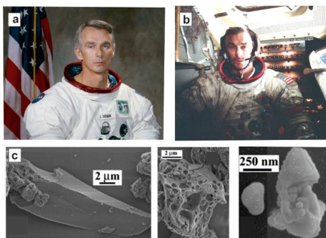
Figure 1. Lunar dust toxicity: a) Jene Cernan in a clean space suit b) suit after moon walk and c) SEM images of inhalable lunar dust
