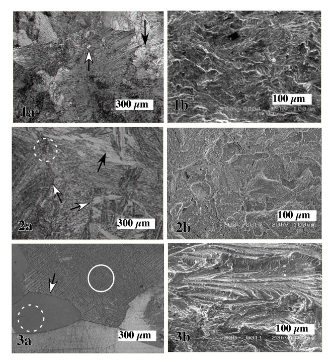
**Fig. 1a.** Optical microstructure of the Pearlitic rail steel with ferrite and cementite lamella (black arrow), & Pearlite (white arrow). **Fig. 1b.** SEM at beginning of the stable crack propagation (LT - RT) region in the pearlitic rail steel.
