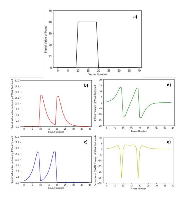
**Figure 1.** (a) Represents the 'time-step' signal value used for testing the algorithm. (b) and (c) represent the 'EWMA Backward' and 'EWMA Forward' respectively. (d) shows the difference between EWMA Forward and EWMA Backward. (e) shows the derivative of the difference computed in (d).
