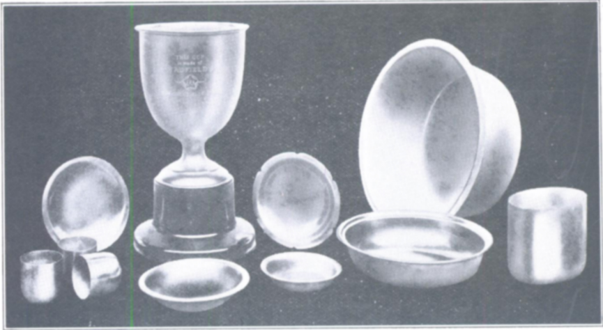
FIG 14 HOLLOW-WARF OF "ERA" NON-CORRODIBLE STEEL Formed by Cold Pressing
