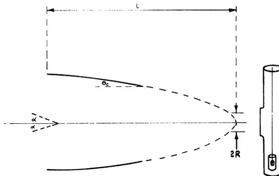
Fig. 4. A grazing incidence X-ray telescope.
