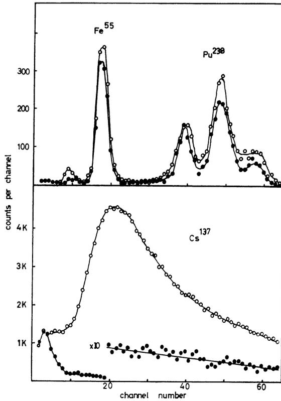
Fig. 3. Pulse shape discrimination with 800 cm<sup>2</sup> counter.
