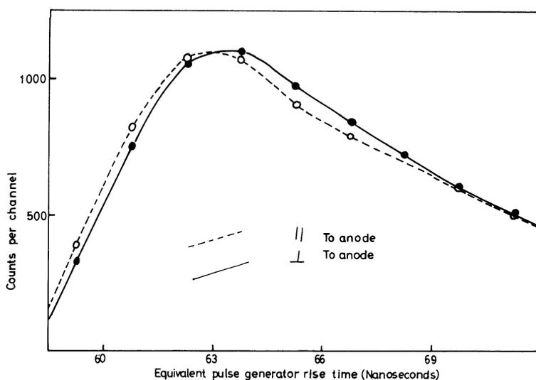
Fig. 7. Pulse rise time distributions for polarized 16.5 keV X-rays.
