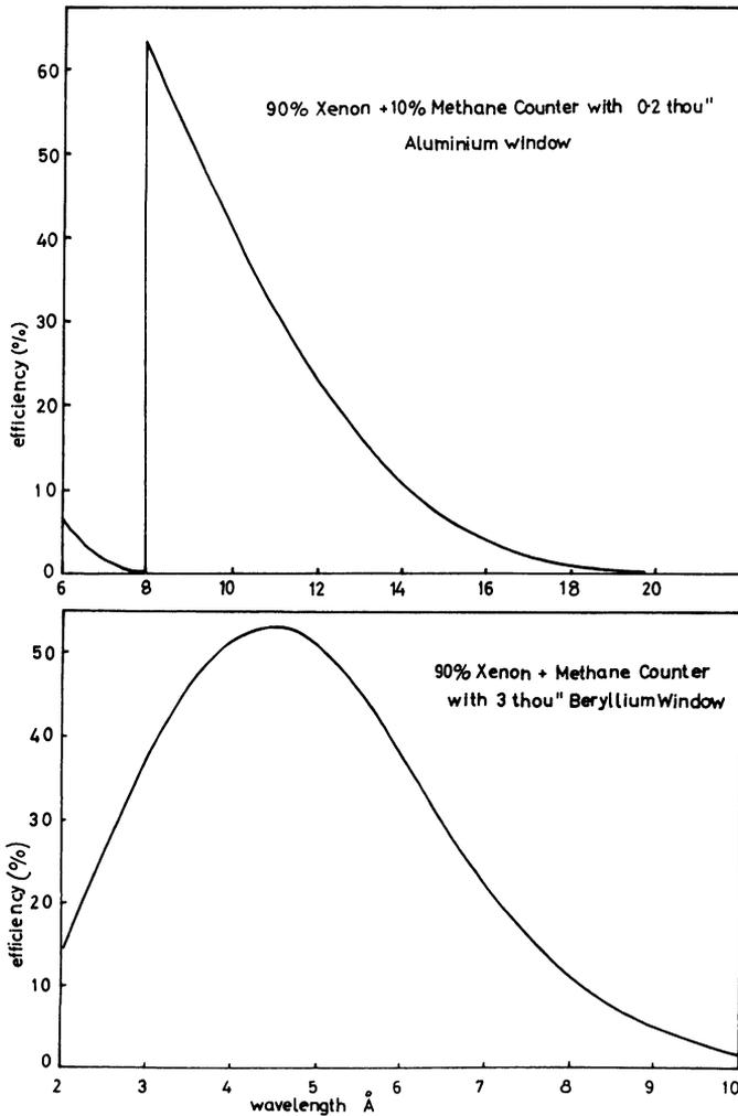
Fig. 6. Detection efficiencies of small volume counters.
