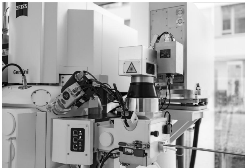
Figure 1. Picture of ZEISS Crossbeam 350 laser with fs laser attached to the airlock.
