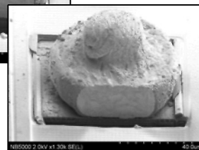
Mill and Monitor: SEM Acquisition while FIB Milling
