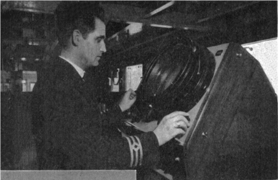
Type 14/12P (True Plot) Display Unit in m.v. 'Tewkesbury'. Of entirely new design this Unit incorporates a 12-inch P.P.I. display with relative motion or true motion presentation. It is suitable for table or deck-pedestal mounting, and can be operated in conjunction with another 12-inch or 9-inch display.
