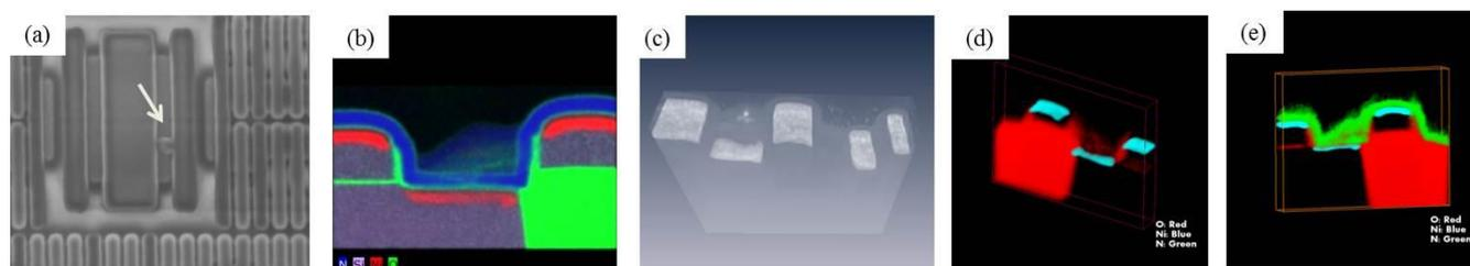
**Figure 1.** (a) Top-down SEM image of the defect location (arrowed); (b) Cross-section EDS elemental map of the defect; (c) STEM tomography voltex visualization of the particle; (d),(e) EDS elemental tomography of the defect.
