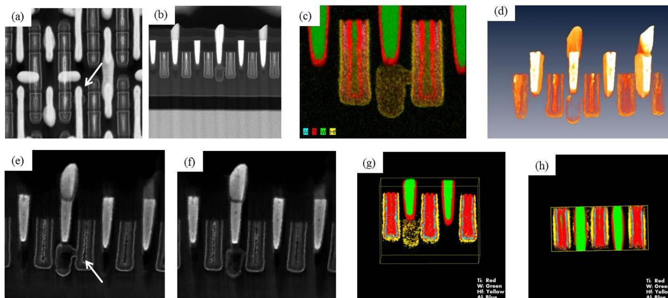
**Figure 2.** (a) Planar-TEM view of the sample; (b) Converted cross-section view of the planar sample in (a); (c) Cross-section EDS elemental map of the defect; (d) STEM tomography voltex visualization of the defect; (e), (f) Reconstructed OrthoSlices of the defect; (g),(h) EDS elemental tomography of the defect.
