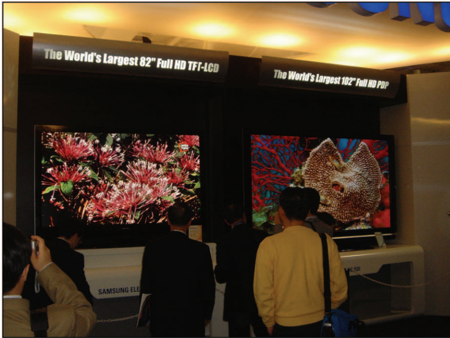
Figure 1. Samsung 82-in. 2-megapixel (Mpx) active-matrix liquid-crystal display (AMLCD) next to a 102-in. 2-Mpx plasma display panel at the Society for Information Display Exhibition in May 2005. The AMLCD has 6 million thin-film transistors in its subpixels and is an example of the state of the art in macroelectronics manufacturing technology for full high-definition (HD) digital television displays. A 100-in. 2-Mpx AMLCD was announced in January 2006 by LG.Philips LCD Co. (Photograph courtesy of D.G. Hopper.)
