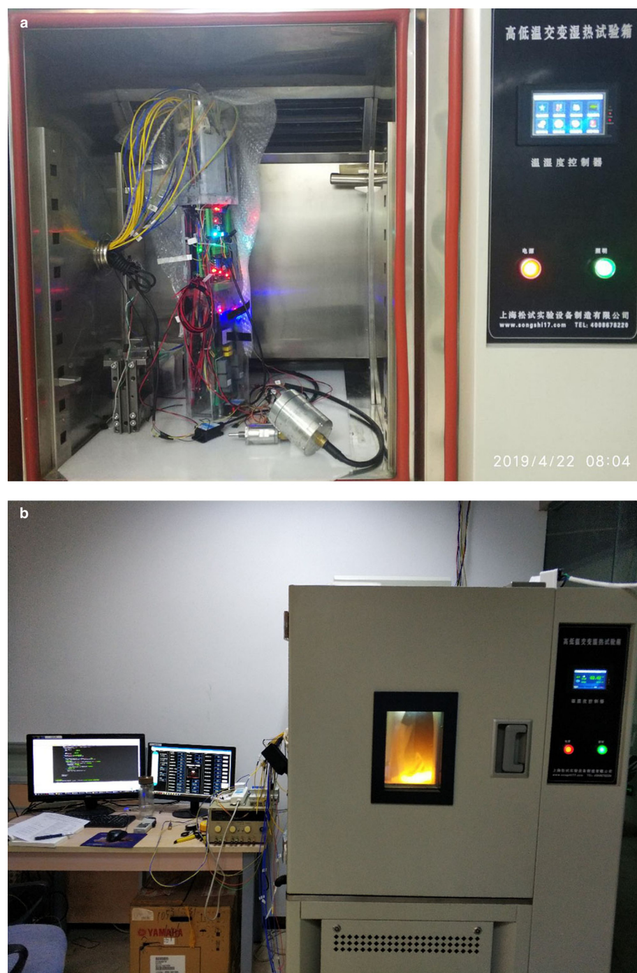
Fig. 21. Low-temperature test of the control system: (a) control system to be tested and the testing environment; (b) ongoing test, and the LED light of the camera system is on.
