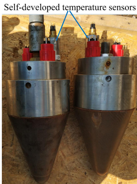
Fig. 11. Temperature sensors and their installation on the thermal heads.
