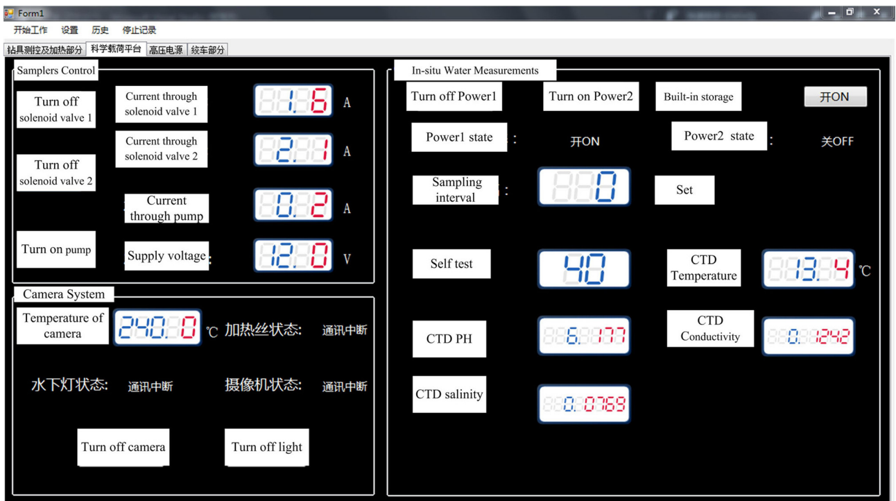
Fig. 20. Control screen of scientific payload system. The left part provides control over the water collection samplers and the camera system. The right part provides control over in situ water measurement sensors and displays the measured water parameters, such as pH, conductivity, temperature and pressure.
