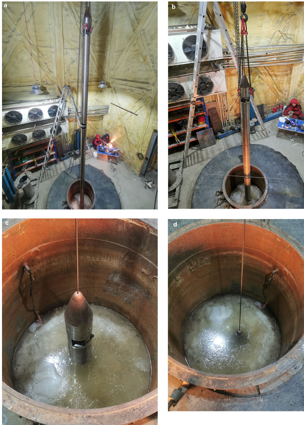
Fig. 24. Drilling of one downward penetration: (a) RECAS starts to drill; (b) probe is mostly halfway into the ice; (c) upper thermal head mostly reaches the ice surface; (d) upper thermal head enters the ice.
