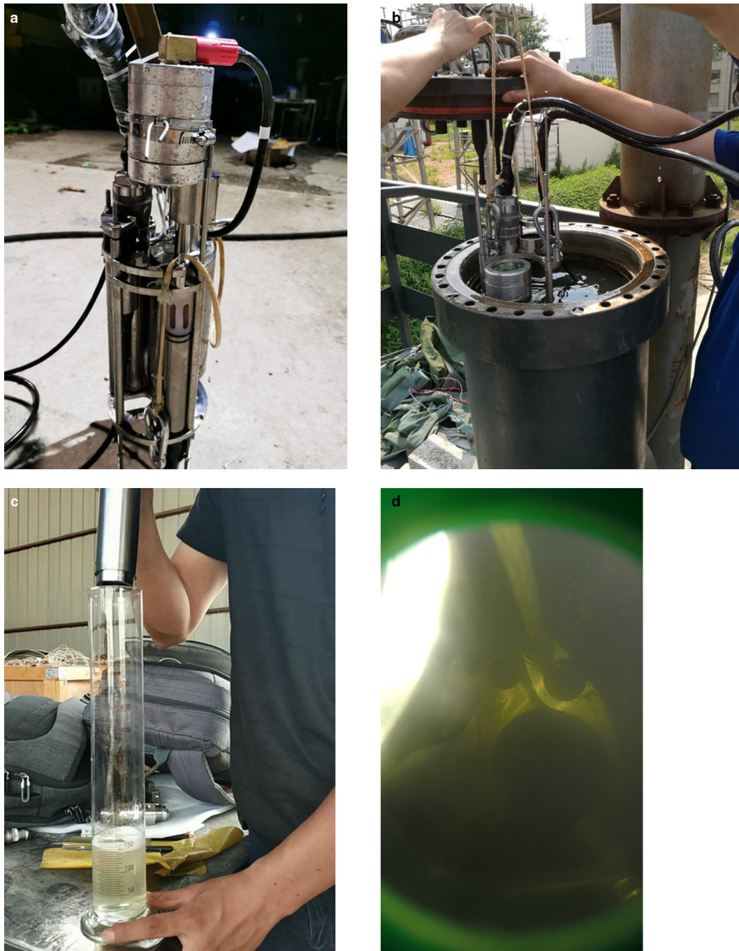
Fig. 22. Tests with the scientific payload system: (a) scientific payload system; (b) pressure tank to simulate underwater high-pressure environment; (c) water sampled in simulated high-pressure environment; (d) picture taken by the camera system.
