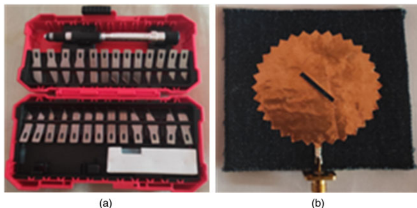
Fig. 2. (a) Scalpel cutting tools set. (b) Front view of the fabricated antenna.
