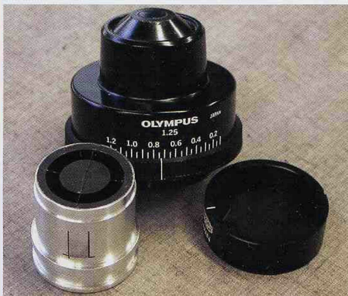
Figure 7-Photograph of the Olympus Abbe condenser and the insert for critical darkfield dispersion staining with the 40X 0.65 NA Olympus objective.
