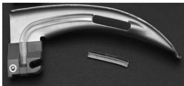
Figure 1. The laryngoscope blade with its fractured fibreoptic light path.
