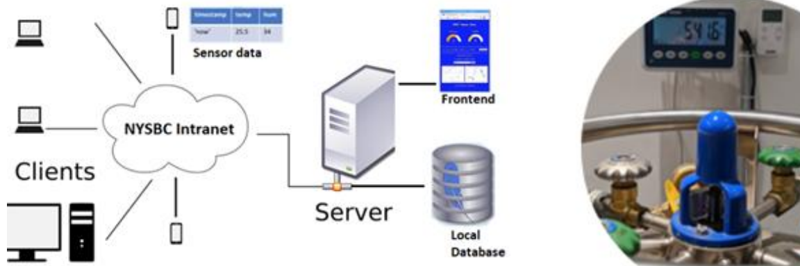
Figure 1. Left: Architecture of sensor monitor network. A range of sensors is available e.g. temperatures, humidity, LN2 weight etc. The software is multi-threading to be responsive to network request and data handling. Right: Typical LN2 tanks for supplying cooling of microscope. Weight is monitored in real time and sent over sensor network. High/low thresholds trigger email alerts to be sent by central server. LN2 consumption is measured and checked against historic numbers and against installed base.
