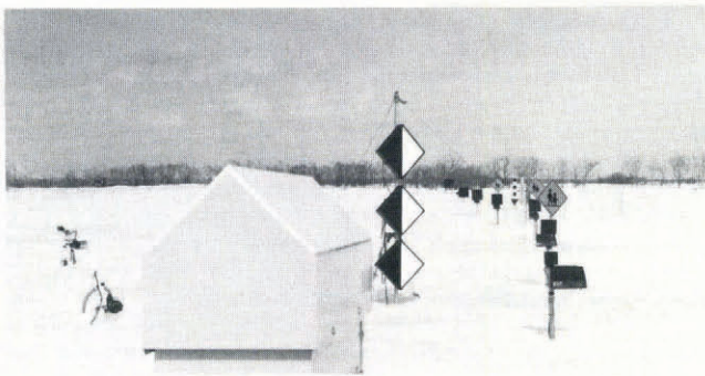
Fig. 2. Three targets installed 30 m from the location of the housing case of the CCD video camera and the optical targets within 0.5° of the visual angle from the observation point.
