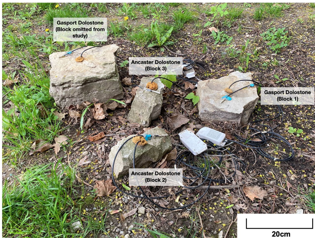
Fig. 5. Experimental set-up for dolostone control blocks maintained in outdoor conditions between December 2020 and March 2021. Thermistors were placed on the block surface and inserted into a borehole 8 cm deep within each block. Dolostones of the Gasport Formation are coarse-grained, fossiliferous and vuggy (block 1), whereas dolostones of the Ancaster Member of the Goat Island Formation (blocks 2 and 3) are relatively fine-grained and contain chert nodules.
