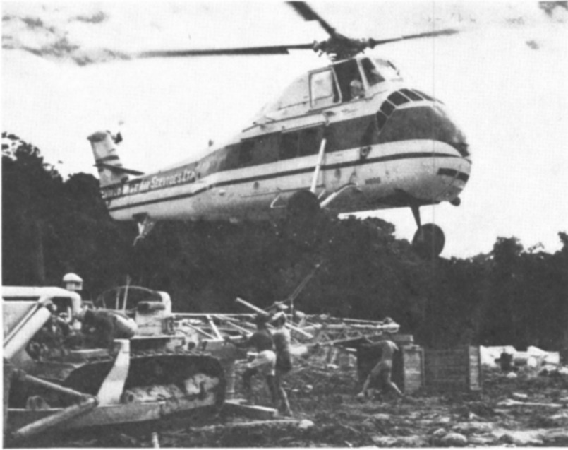
AIR LIFT OF OIL DRILLING EQUIPMENT IN PAPUA Helicopter lowering a crane-jib into position on a caterpillar tractor at Sireru rig-site
